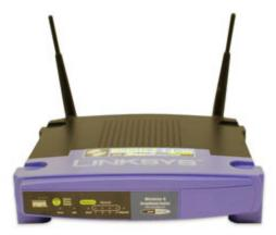
A **router** is a hardware device that allows you to connect **several computers** and **other devices** to a single Internet connection, which is known as a **home network**. Many routers are **wireless**, which allows you to create a **home wireless network**, commonly known as a **Wi-Fi network**.
